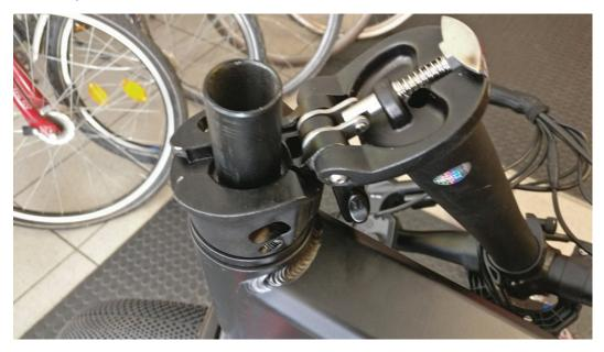
8. The length of the steerer tube of the stock fork is 182 mm (+- 1 mm).
