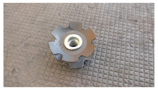
14. Use a star nut driver to put the nut in place
