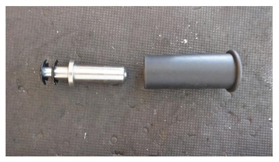
15. Hit the driver with a hammer until the star nut is in place
