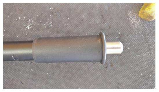
16. The steerer tube now has a thread for mounting
