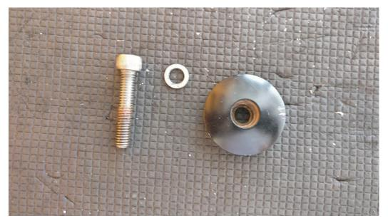
19. Screw the ahead bolt into the star nut
