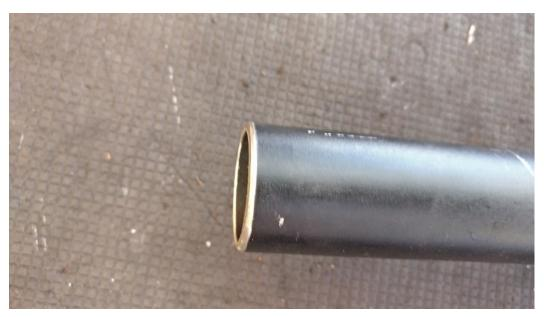
13. The new fork came with a star nut that needs to be driven into the steering tube.
