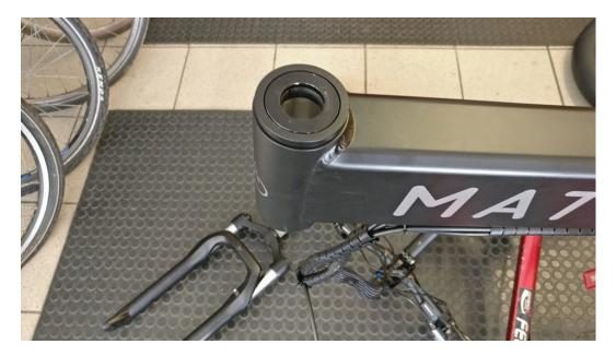
4. As you can see the new fork has a longer steering tube (in this case 220 mm) and a slightly longer travel (15 mm).
