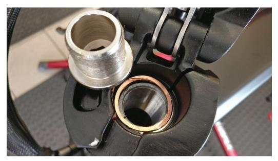
3. Remove the stem by loosening the two bolts. You can now remove the fork. Keep the rest of the headset untouched, you will reuse it with the new fork.
