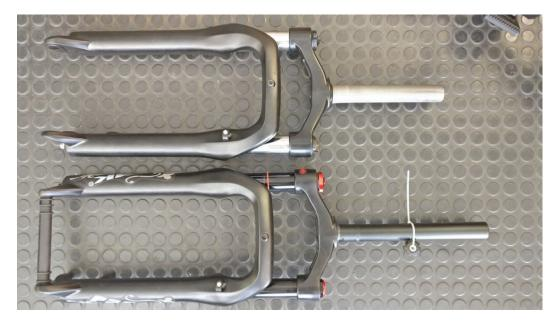
5. You now have to remove the lower bearing shell from the old fork. There is a small notch on one side to ease the removal. Be careful not to damage the bearing shell and use a knife or small screwdriver if needed.
