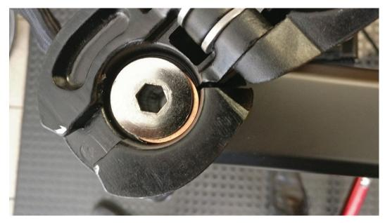
1. Fold the handlebar stem to reveal the headset
