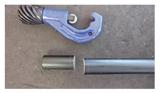
11. Deburr and file a light chamfer into the tube for easier mounting
