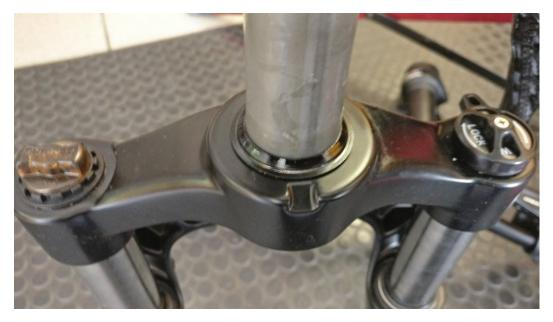
6. Put the bearing shell on the new fork.
