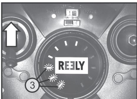
When the control lever for the pitch function is back in the lower position, the four LEDs in the upper area of the LED display ring (2) will go out, and the three LEDs in the lower left of the LED display ring (3) are lit continuously.
