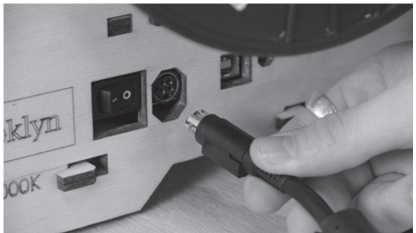
Step 10. Make sure the power switch is in the OFF position when you connect the power cable.
