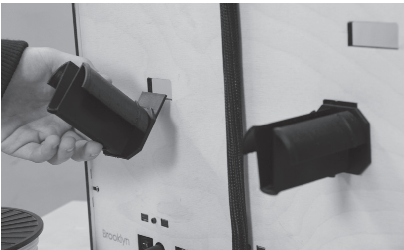
Step 8. Spool holders fit into the slots as shown.
