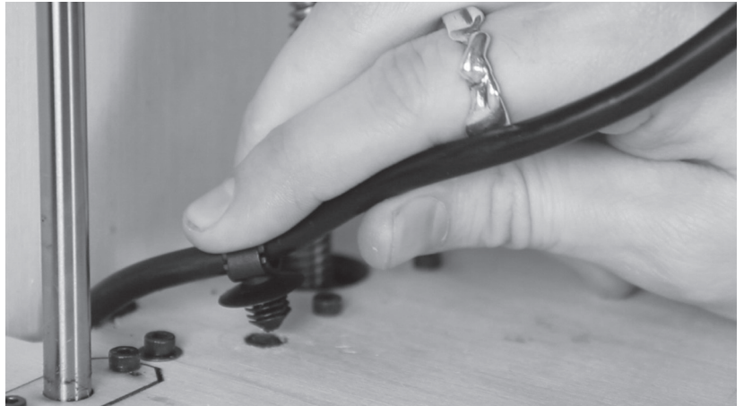
Step 5. Snap the cable clips into place.
