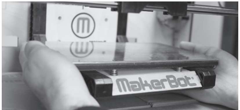
Step 4. Grasp the platform firmly on both sides and lift with gentle pressure.
