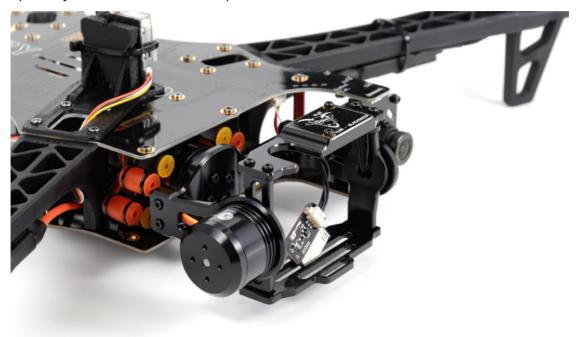
**Important:** Avoid rotating the gimbal multiple full turns on the tilt-axis. This puts tension on the IMU cable which in turn introduces counter-forces and interferes with the normal operation of the gimbal.
