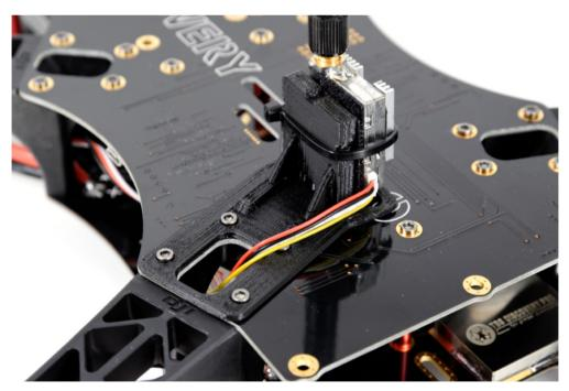
• Powerful video transmitters, such as the ImmersionRC 5.8GHz 600mW or more powerful VTx, must be powered directly from the bottom frame (small +/- pads) to avoid overdriving the CORE. Test this a few minutes on the ground and verify that the CORE does not reboot which indicates a thermal protection shutdown/overcurrent.
