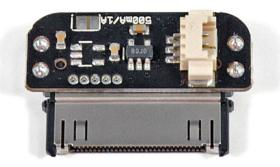
(Advanced users only) There is even a component you can add on the board to be able to change the charging rate from 0.5A to 1A continuous. To enable faster charging, solder a dab on the two pads on the back-side labeled "500mA/1A" and order the IC NCP380HSN05AAT1G from Mouser or Digi-Key. Solder the IC to the unoccupied pads on the adaptor board (adequate soldering skills needed.)
