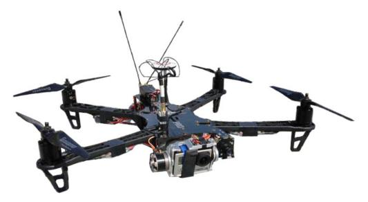
By implementing the wiring into the frame, the copter is easy to build and outperforms similar quads in terms of FPV range and video link quality. The DJI Flamewheel arms as predetermined breaking point protect your electronics and are easily replaceable in the field.
