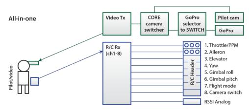
• **Dual operator** - Introducing a separate video operator for the gimbal roll and tilt control requires one additional video transmitter and R/C receiver. Disable the video switcher, cut the trace between the two "GP OUT SEL" jumper pads and solder the left pad to the middle.
