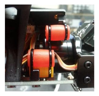
Continue assembling the rest of the DISCOVERY PRO frame and at the end of the build attach the gimbal assembly to the front of the frame and plug in the 3 connectors. Align and fasten the four screw holes on the mounting brackets. Adjust the gimbal so that it is parallel and true to the frame. The arms and motors should not be tilting at an angle, looking from the side. Use the sliding position holes on the bottom plate to make the final adjustment.
