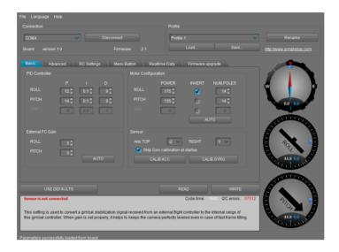
If you want to apply updates and make adjustments to the gimbal, download the SimpleBGC and driver package (<u>www.simplebgc.com</u>), plug in battery power, and connect the DISCOVERY PRO to a Windows computer via a micro USB cable (e.g., from the NAZA-M or a mobile phone.) Extensive details of the brushless controller is available in the SimpleBGC manual. The TBS Profiles can be downloaded from the product page.
