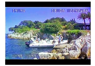
• The OSD is enabled by default, to disable it completely hook up video and press the "ENTR" button on the top plate for 4-5 seconds, toggle to the "OSD" menu and select "OSD OFF".
