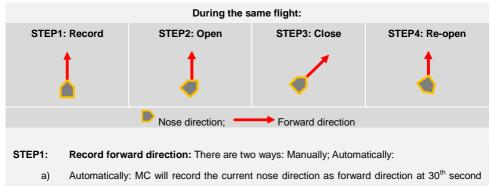
after you power on the multi-rotor. And LED will blink oquickly if recording is successful.
